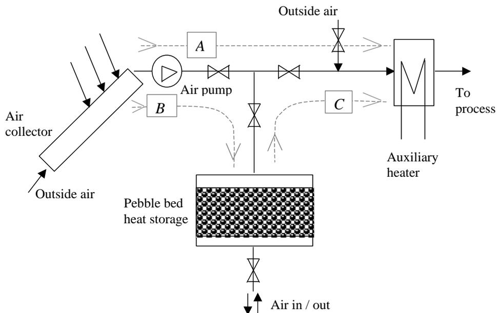
There are three basic modes of operation of these systems. The dashed lines indicate the directions of airflow for each of these modes, A, B, and C.
