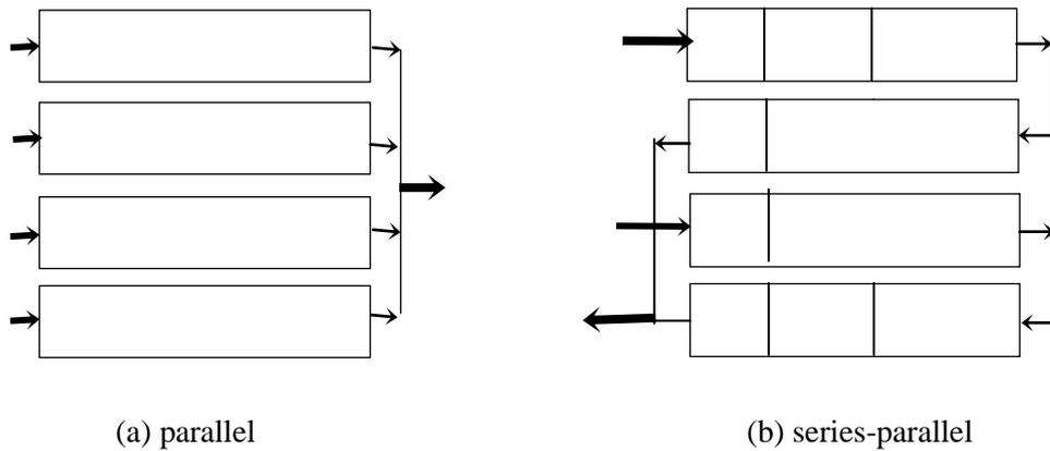
Neglecting the entry length effects in long collector modules, the series-parallel combination essentially works as a parallel combination where the collective thermal performance of modules connected in series is similar to one lengthy module making up the total length.
