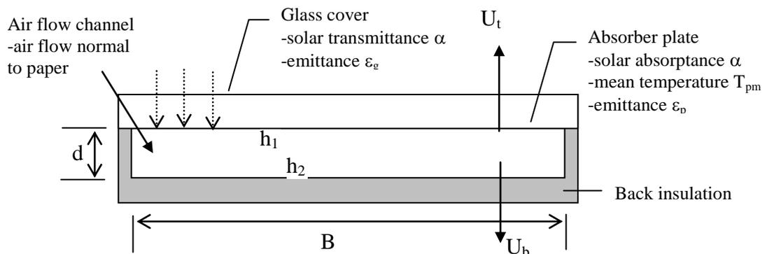
Following the analysis of Niles et.al. and Duffie and Beckman, the performance of a solar air-heating collector (Figures A1 and A2) can be given by;
